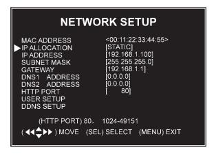
By default, the DVR IP mode is set to Static. Changing the Static to DHCP, will cause the DVR to automatically retrieve an IP address from the connected router. Unless your network requires a static IP address, leave the DVR IP Allocation set as DHCP.
